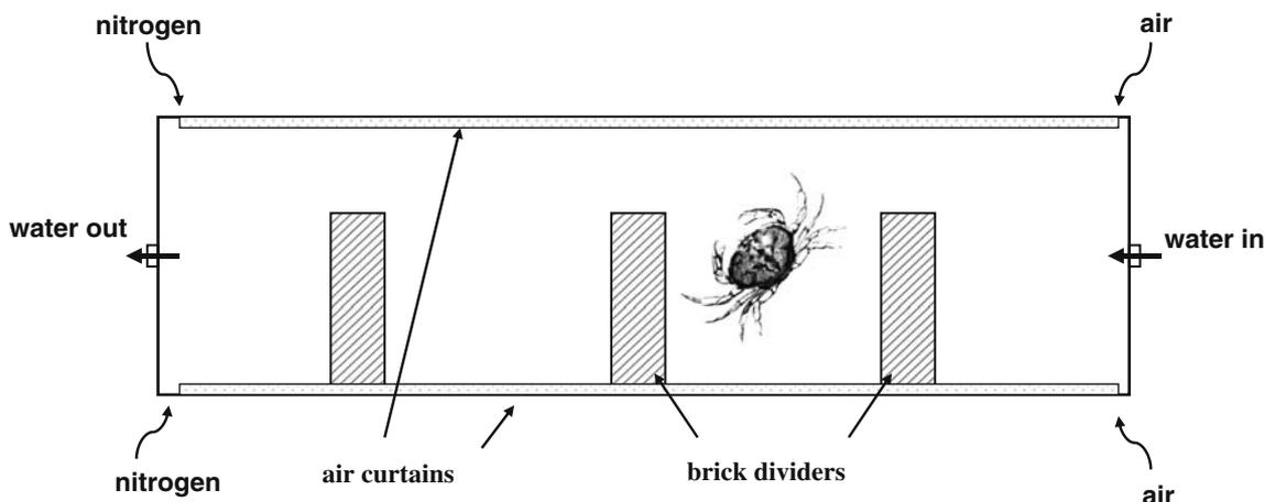
**Fig. 1** Diagram of apparatus used for oxygen gradient experiments. A constant flow of seawater ( $2.5 \text{ l min}^{-1}$ ) maintained the salinity at 31–32‰ and the temperature at 10–12°C. Separate air curtains placed along the length of the tank allowed varying mixes
